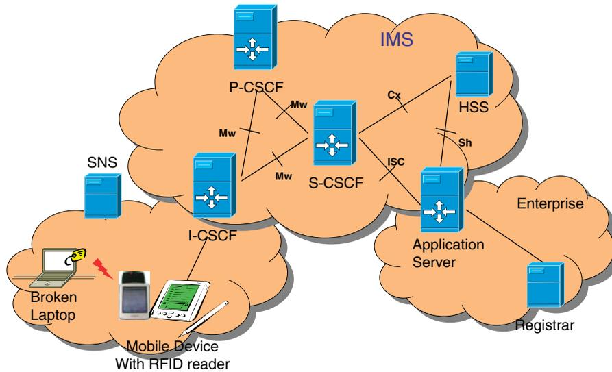
Figure 5. Mobile RFID architecture based on IMS.
