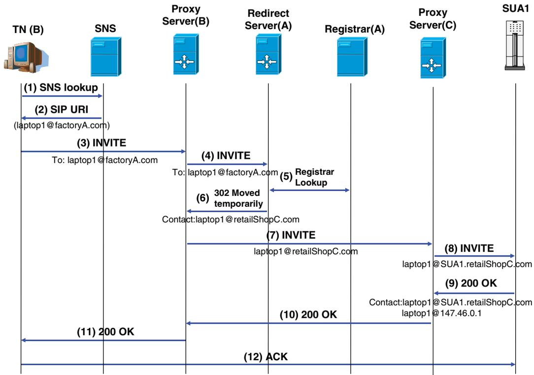
Figure 4. Location tracking procedure in SRMS.
