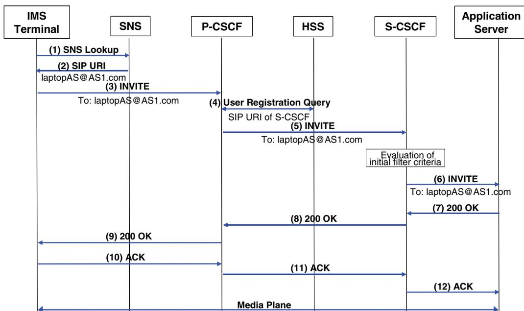
Figure 6. Mobile RFID procedure in SRMS.
