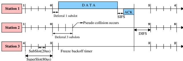
Fig. 1. Slot structure for two-phase collision avoidance
