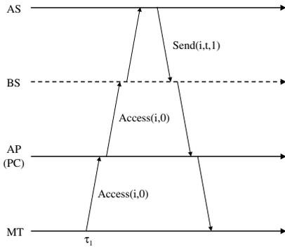
Fig. 2. P-PER operation: There are no cached objects both in the MT and the PC.
