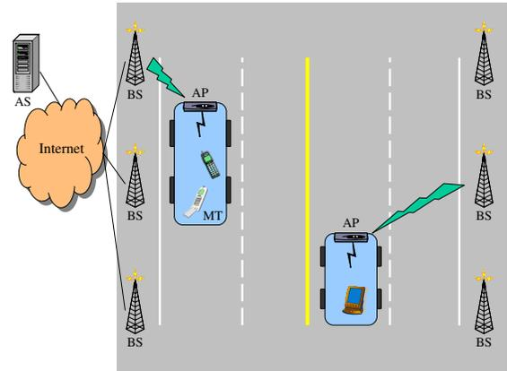
Fig. 1. Wireless data access in ITS-based networks with multi-hop wireless links.
