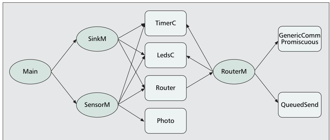
■ Figure 4. Sensor node structure.
