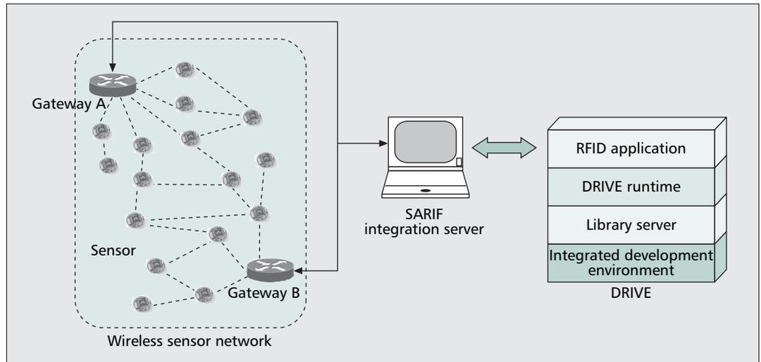
■ Figure 3. SARIF prototype architecture.
