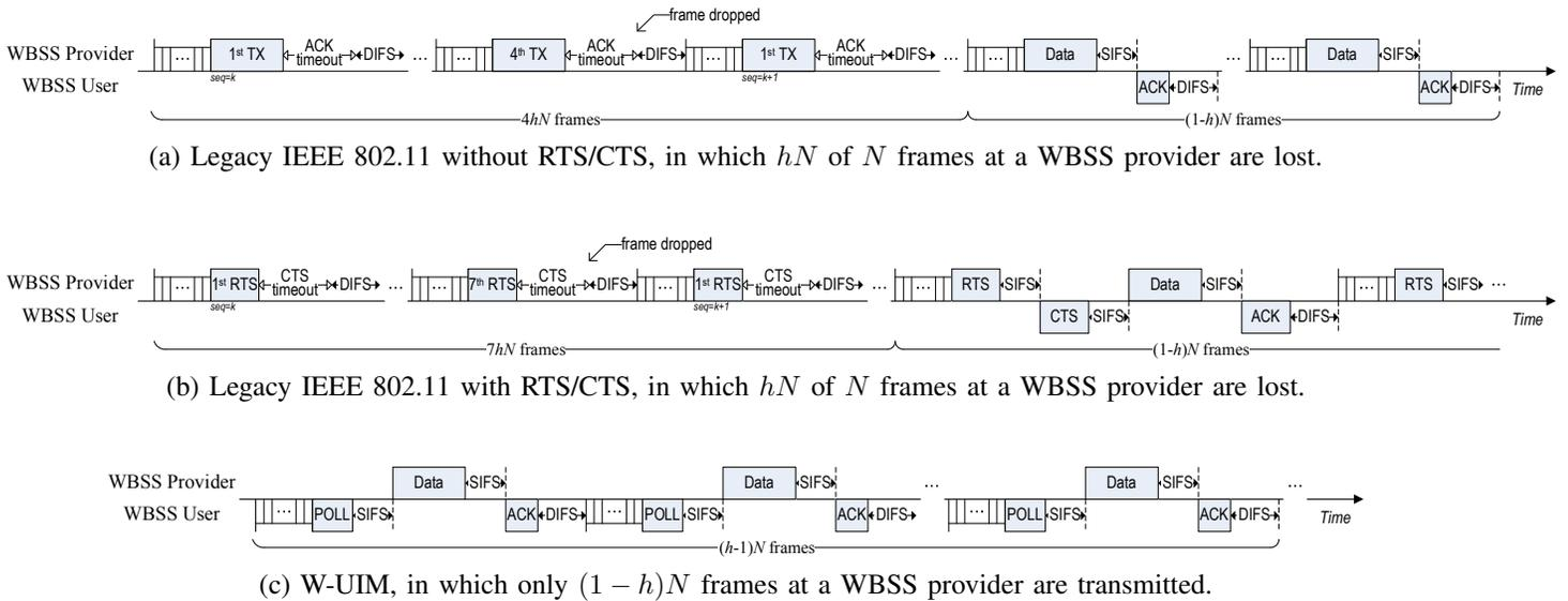
Fig. 4.  $N$  frame transmissions when  $hN$  WBSS users move away.
