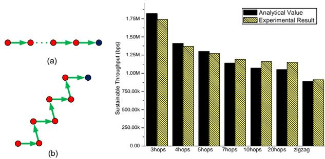
Fig. 4. Topology and Single flow results.
