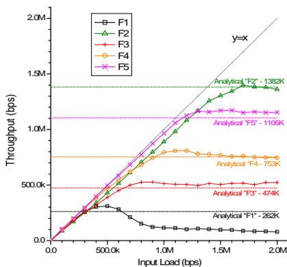
Fig. 9. Results of Scenario with Multi-Flows and Multi-Gateway
