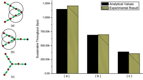
Fig. 7. Topology and simulation results.
