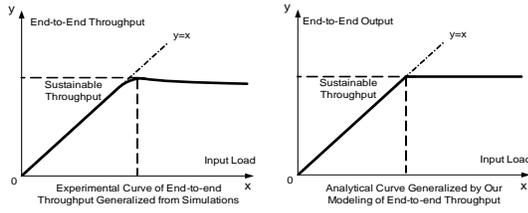
Fig. 3. Average Throughput of All Flows (Simulation on the left and Modeling on the right)
