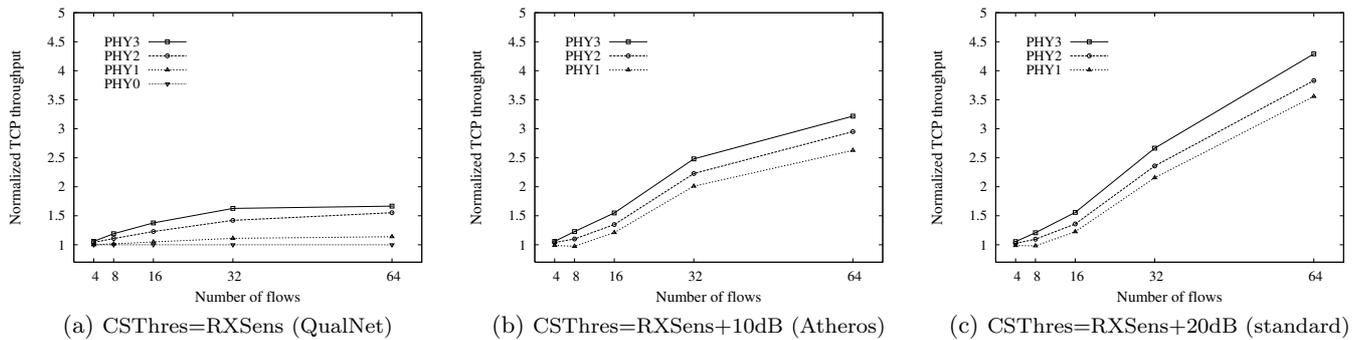
**Figure 3: Aggregate TCP throughput of indoor propagation model with different CStHres settings. Normalized by PHY0(CStHres=RXSens).**
