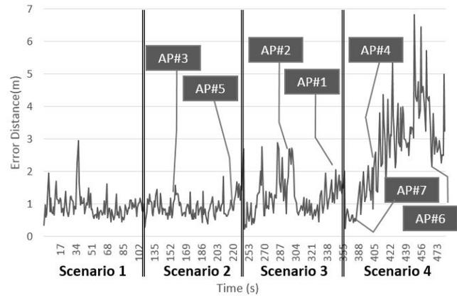
**Figure 6:** Localization errors are plotted for each different scenario. Each AP number is to indicate when it is broken down.
