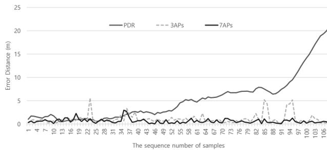
**Figure 5:** How localization error is propagated is shown depending on the number of available APs.
