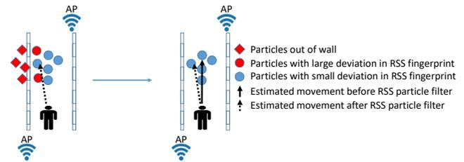
Figure 2: The particle filtering algorithm is compensated by the fingerprinting data
