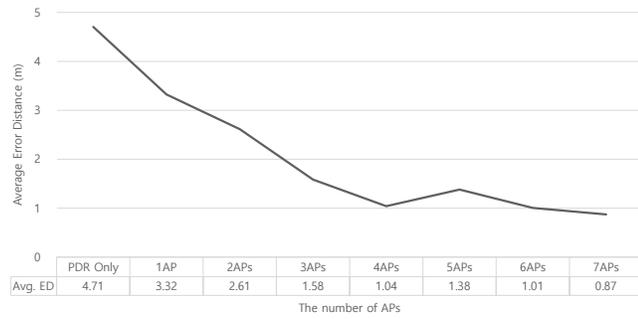
**Figure 4:** We plot the localization performance with the partially available infrastructure. The localization error is decreased as the number of available APs increases in the simulation.
