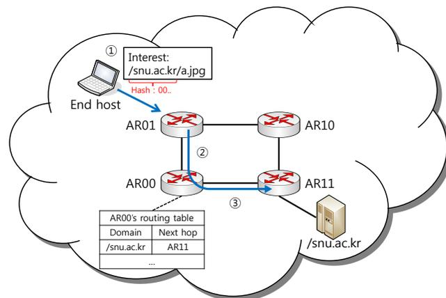
Fig. 1. Routing interest packet in intra-domain routing
