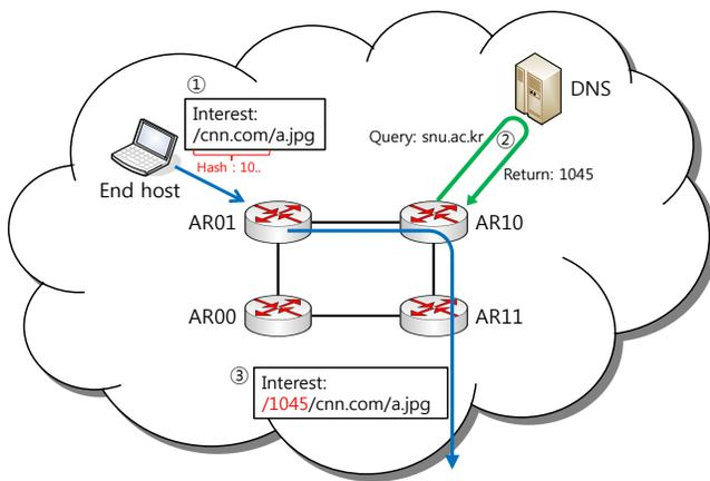
Fig. 2. Routing interest packet in intra-domain routing
