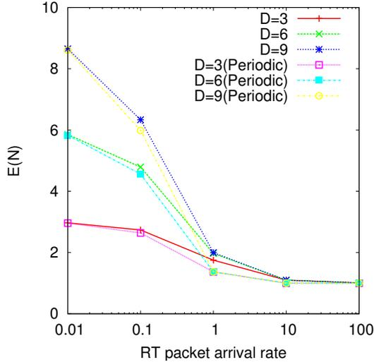
Fig. 3. Average aggregation degree vs. RT arrival rate.
