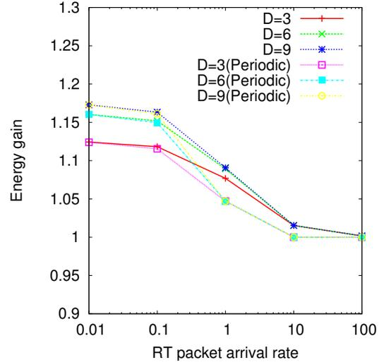
Fig. 4. Energy gain vs. RT arrival rate.
