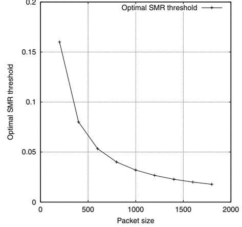
Fig. 5. Optimal SMR threshold as a function of packet size
