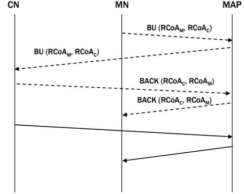
Fig. 2. Packet delivery with the GRO scheme
