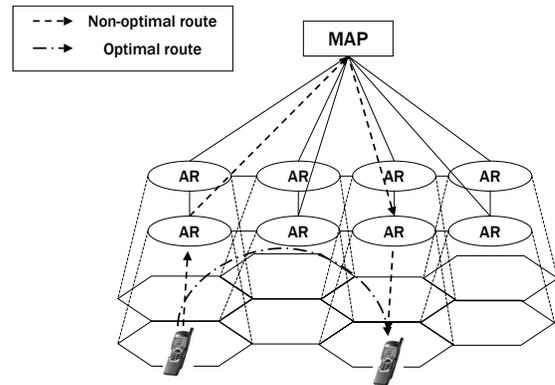
Fig. 1. Non-optimal routing problem in HMIPv6 networks
