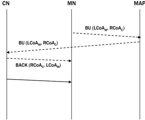
Fig. 3. Packet delivery with the LRO scheme: Uni-directional
