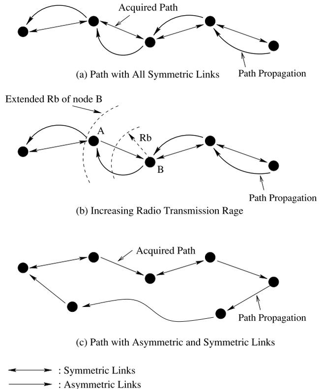
Fig. 1 Acquiring a path at routing protocol.
