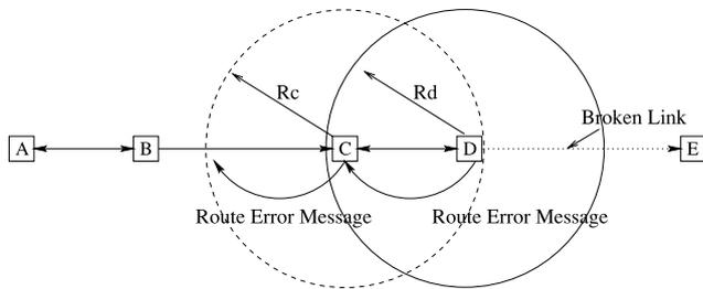
**Fig. 6** The case where Route Error Message cannot be propagated to the source node.
