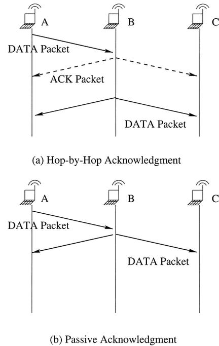
Fig. 2 Two link level approaches for route maintenance and flow control.
