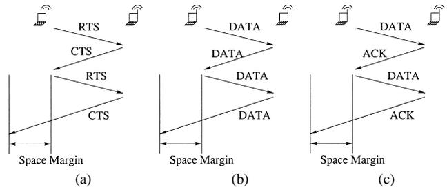
**Fig. 7** Some relationship with signal strength: (a) IEEE 802.11 based, (b) passive acknowledgment and (c) DSR-specific acknowledgment.
