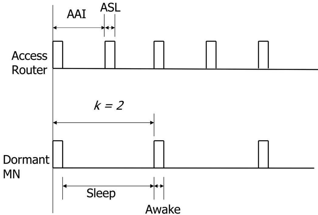
Figure 4: Power save timing diagram. The access router broadcasts agent advertisement (AA) message once per AA interval (AAI). Advertisement slot length (ASL) is the time during which the AR may broadcast an AA. The idle MN wakes once in maximum paging interval, i.e.,  $\kappa$  times the AAI, to check if it has a paging alert.
