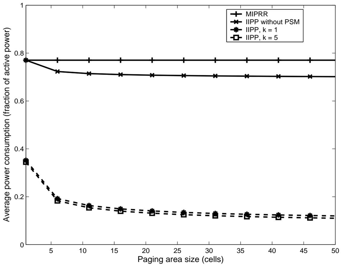
Figure 7: Average power consumption of a mobile node versus paging area size.
