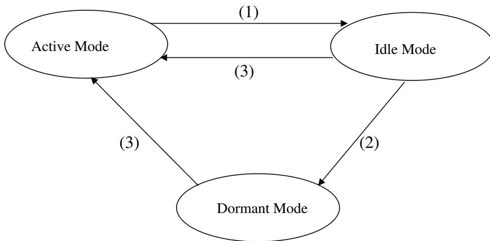
Figure 2: Modes of an IIPP mobile node. The mobile node remains in active mode as long as it is sending or receiving data packets. When it finishes the data session it enters idle mode, as shown by arrow (1). After an active timeout in idle mode, the mobile node enters dormant mode, arrow (2). The mobile node enters active mode from idle mode or dormant mode when it receives a paging request or it has data packets to send or it moves to a new paging area, arrow (3).
