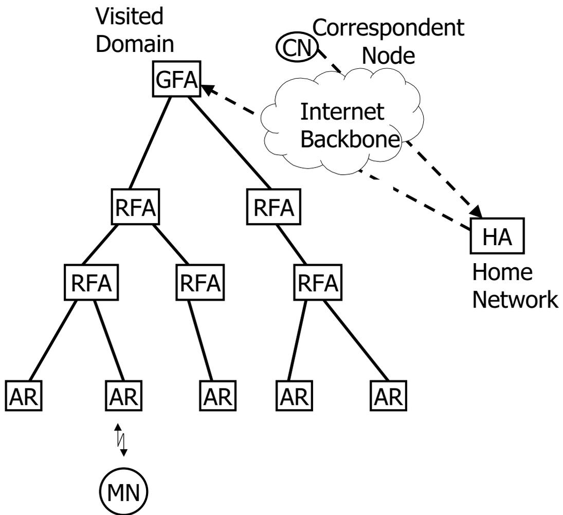
Figure 1: Reference architecture of IIPP.
