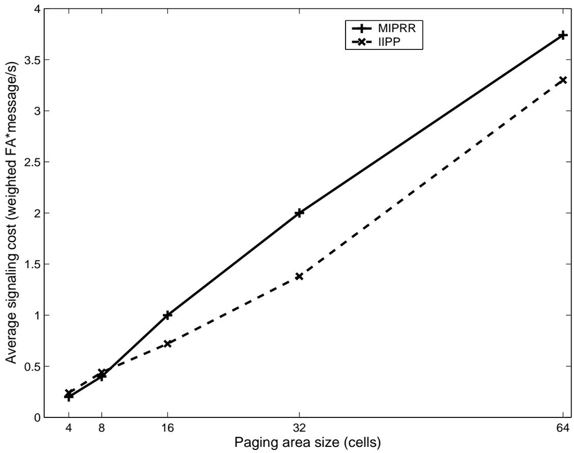
Figure 11: Signaling cost versus paging area size (simulation).
