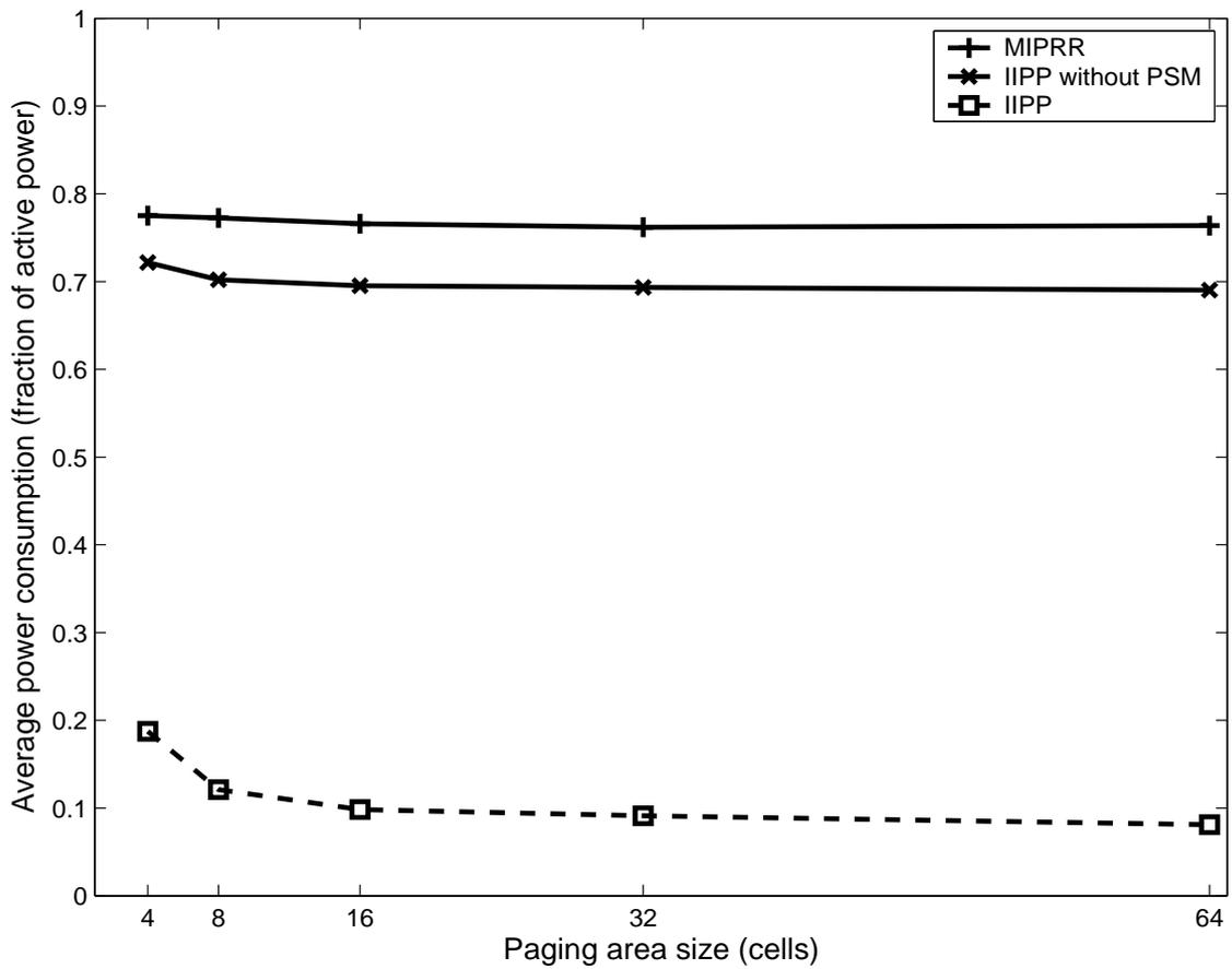
Figure 10: Average power consumption versus paging area size (simulation).
