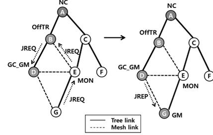
Fig. 2. Join Procedure of MTM: Node G Join
