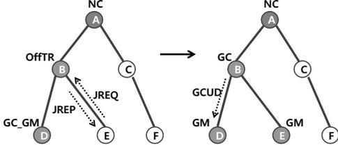
Fig. 1. Join Procedure of Basic Tree: Node E Join
