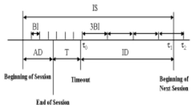
Figure 1 The Timing Diagram in the Adaptive Power Saving Mechanism
