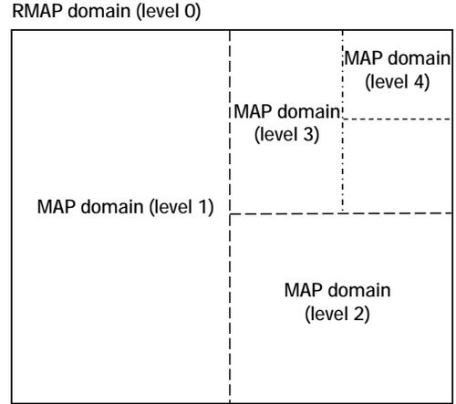
Fig. 2. Rectangular cell configuration in multi-level HMIPv6
