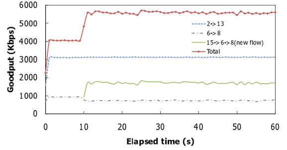
Fig. 5. The total throughput and the throughput of each flow with FIRM<sup>+</sup>.
