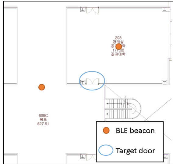
Figure 6. Locations of two BLE beacons and the target door are shown in the floor map.
