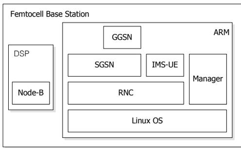
**Figure 3. Architecture of femtocell base station. Its components include Node-B, RNC, SGSN and GGSN.**
