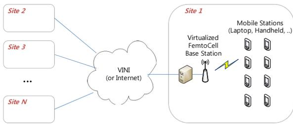
**Figure 1. Cell-Lab sites can be connected via Internet, and will be integrated with wired testbed e.g. VINI.**
