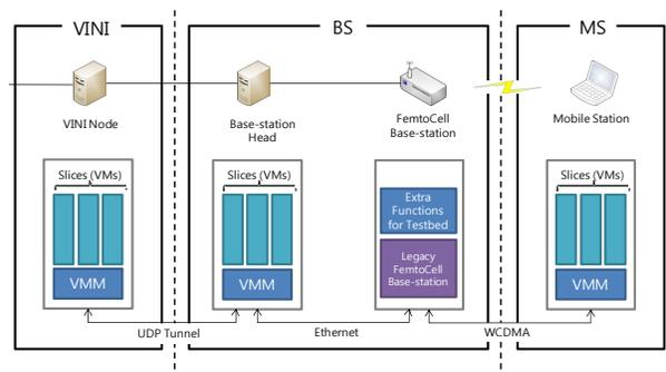
**Figure 2. Cell-Lab implementation scenario. Separate base station head virtualizes femto-cell base station.**
