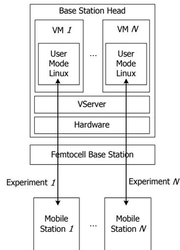
**Figure 4. Cell-Lab reference model. VServer runs on the base station head.**
