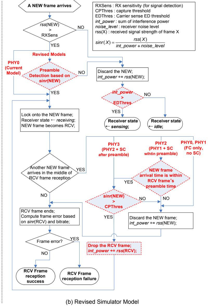
Figure 9: Simulator model flow charts.
