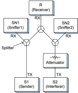
Figure 3: Testbed topology for the capture effect.
