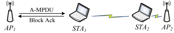
Figure 1: Experiment setup designed for inferring the reason of frame losses from AP_1 to STA_1 . Block ACK bitmaps are collected at AP_1 .
