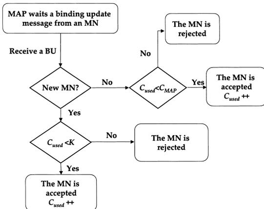
Fig. 2 Proactive load control procedure.
