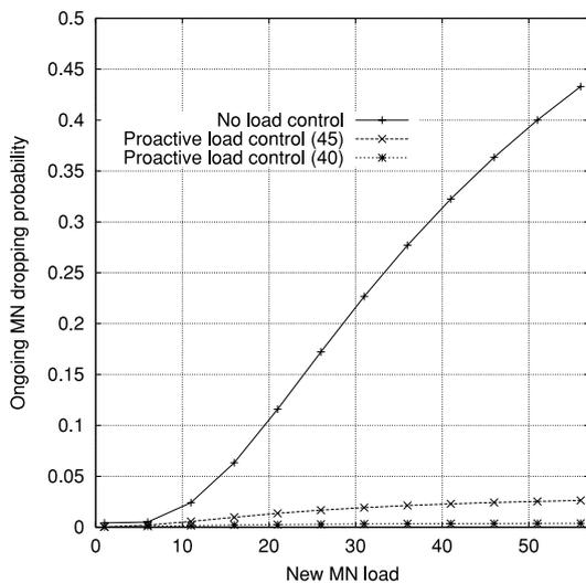
Fig. 6 Ongoing MN dropping probability as a function of new MN load.
