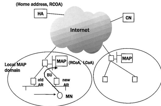
Fig. 1 Basic binding update procedure in HMIPv6.
