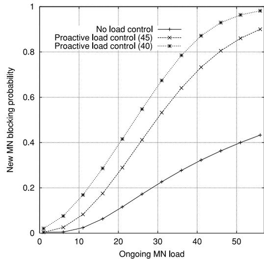
Fig. 7 New MN blocking probability as a function of ongoing MN load.
