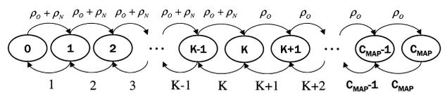
Fig. 4 Markov chain model for the proactive load control scheme.
