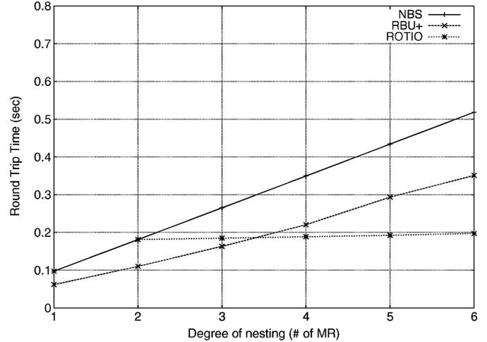
Fig. 11. The effect of the degree of nesting on RTT.
