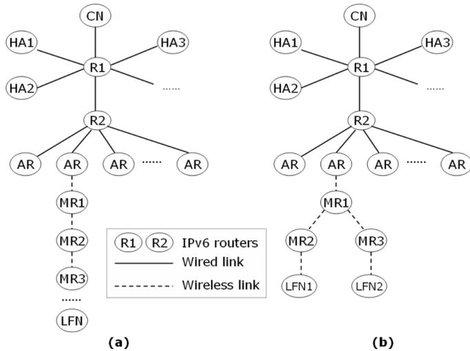
Fig. 10. Network topology for the ROTIO simulation.
