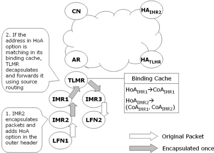
Fig. 7. Route optimization between LFNs in the same mobile network.
