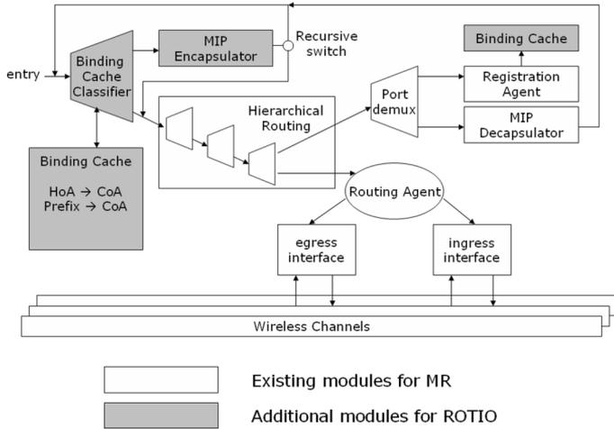
Fig. 9. MR node architecture for ROTIO in NS2.
