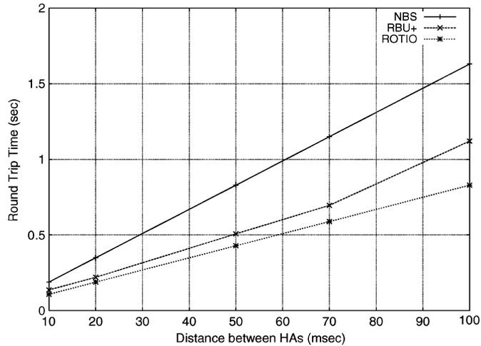
Fig. 12. How the RTT changes as the distance between HAs increases.
