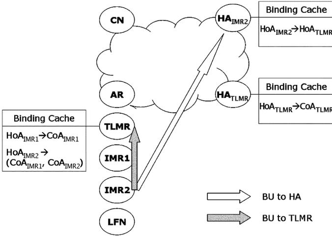
Fig. 4. Binding update of IMR2 in ROTIO.
