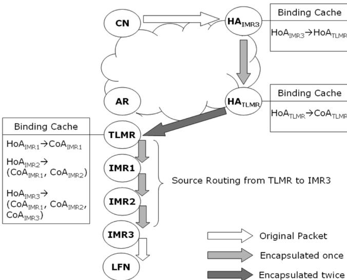
Fig. 5. Route optimization from the CN to the LFN.
