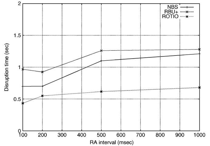
Fig. 14. The disruption time while handoff as the RA interval increases.
