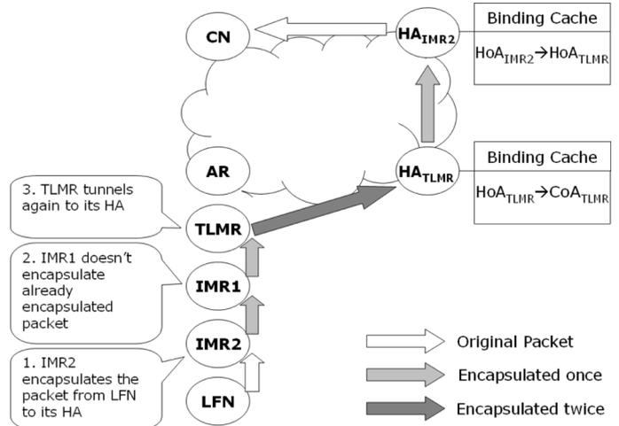
Fig. 6. Route optimization from the LFN to the CN.
