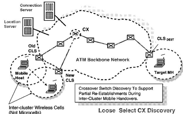
Figure 2. A WATM network structure showing the CX switch.
