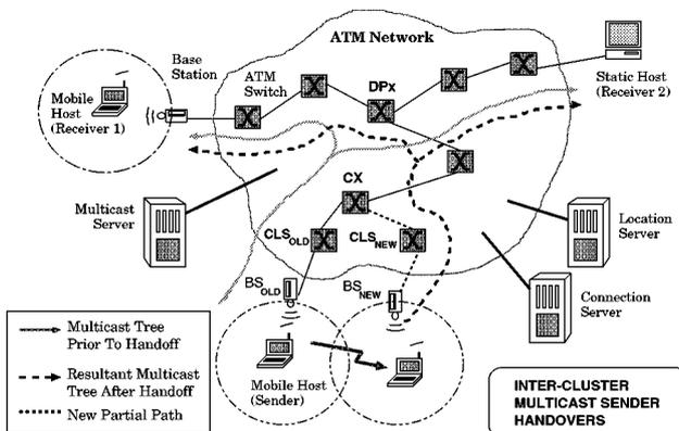
Figure 5. Reconfiguration of the multicast tree after a sender’s handover.
