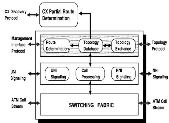
Figure 1. Interaction of CX discovery with P-NNI routing.
