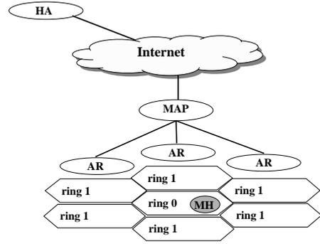
Fig. 1. IP-based cellular architecture based on HMIPv6.
