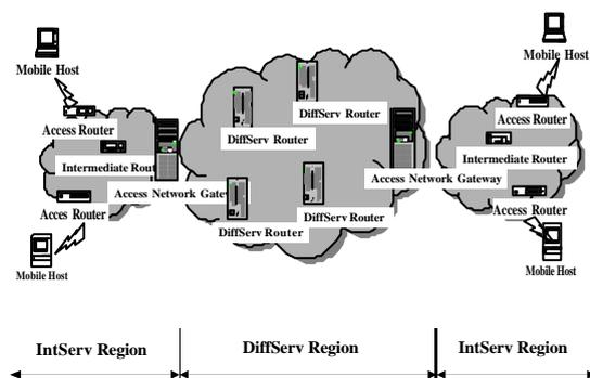
[Figure 1: End-to-End QoS Architecture]
