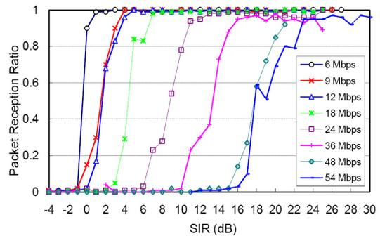
**Fig. 3. PRR of link B→C with interferer A for multiple 802.11a PHY rates. Only B carrier senses A, not vice versa.**
