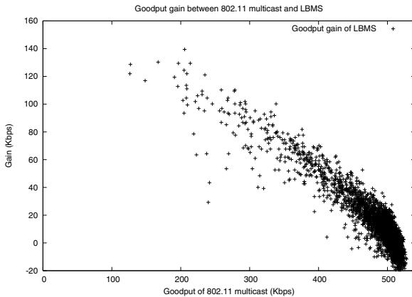
Fig. 5. Goodput gain between IEEE 802.11 multicast and LBMS, with 5 multicast receivers and no background source.
