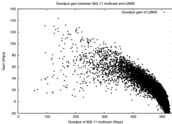
Fig. 7. Goodput gain between IEEE 802.11 multicast and LBMS, with 20 multicast receivers and no background source.
