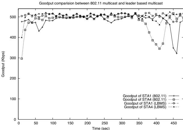
Fig. 4. Goodputs of STA1 and STA4 in LBMS and legacy multicasting with the same mobility scenario. Each point is the goodput for 10 seconds.
