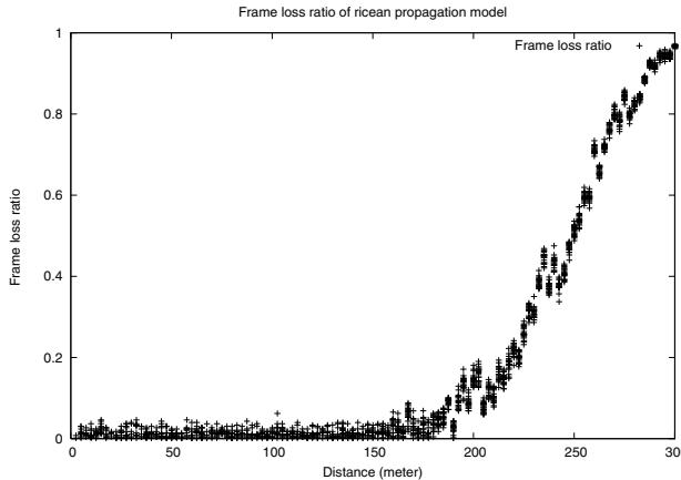
Fig. 3. Frame loss rate changes as the distance between an AP and a STA increases.
