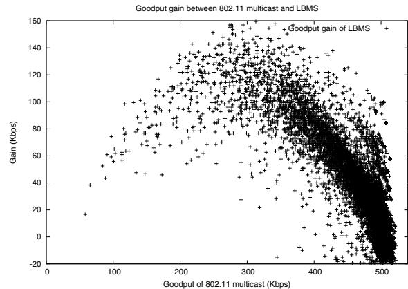
Fig. 8. Goodput gain between IEEE 802.11 multicast and LBMS, with 20 multicast receivers and 5 STAs with background traffic.
