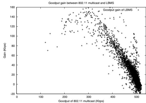
Fig. 6. Goodput gain between IEEE 802.11 multicast and LBMS, with 5 multicast receivers and additional 5 STAs with background traffic.
