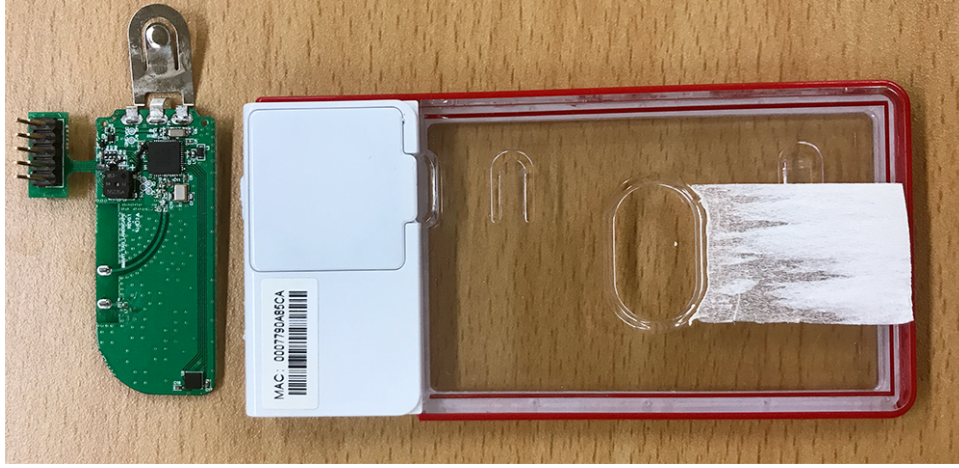
Fig. 5. The implemented localization IoT device, in the form of an ID card on which a small board is mounted. The board contains a magnetometer, an accelerometer, and a BLE interface.
