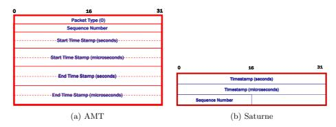
Fig. 1. Probe Packet Format
