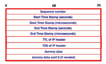
Fig. 3. Probe Packet Format of STAR
