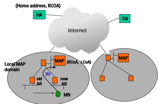
Fig. 1. HMIPv6 Architecture
