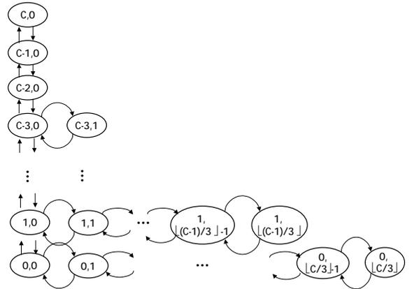
Fig. 3. Markov chain model for the extended HMIPv6 ( $m=3$ )
