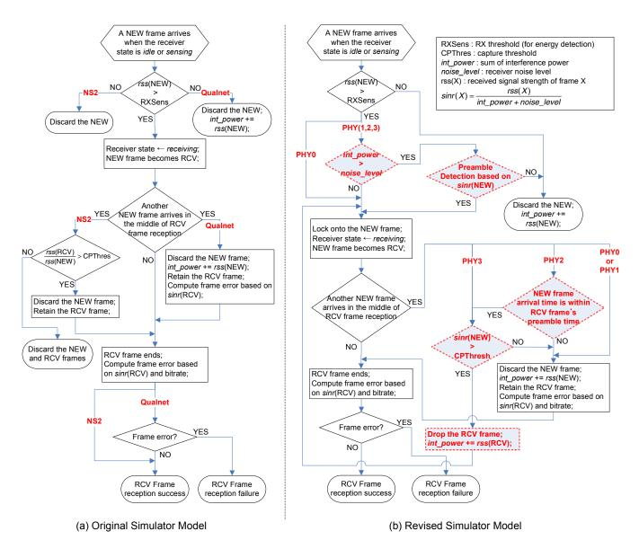
Figure 3: Simulator model flow charts.
