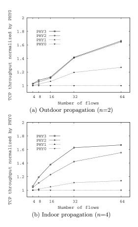
Figure 4: Average aggregate TCP throughput normalized by PHY0.
