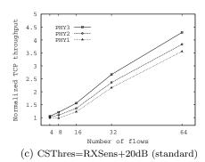
Figure 8: Aggregate TCP throughput of indoor propagation model with different CSThres settings. Normalized by PHY0(CSThres=RXSens).
