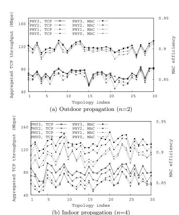
Figure 7: TCP throughput and MAC efficiency (16 flows).
