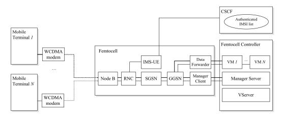
Fig. 1. Overall testbed architecture
