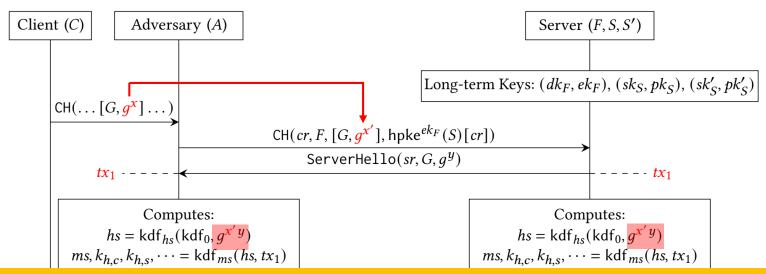
Main idea: Encrypt the whole ClientHello destined for the backend server (inner) and bind it with the ClientHello for the Client-Facing server (outer)
