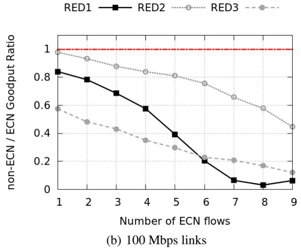
**Figure 6: Unfairness between ECN and non-ECN flows for several flow-type mixes and RED parameter sets, given a constant number of 10 flows. In all parameter sets, the unfairness becomes larger when there are fewer remaining non-ECN legacy flows.**
