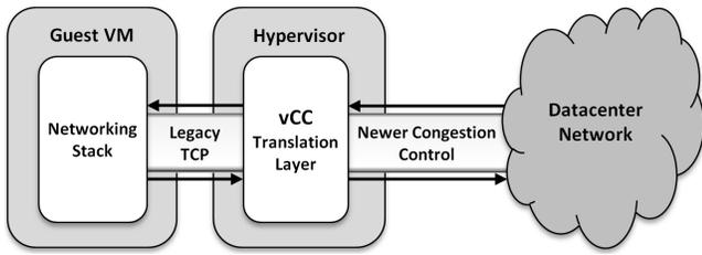
**Figure 2: High-level illustration of vCC (virtualized congestion control). The vCC translation layer sits in the hypervisor, where it translates the guest’s legacy congestion control to a target congestion control algorithm.**
