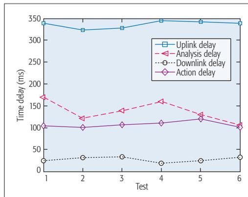
Figure 5. Evaluation of interactive end-to-end delay.
