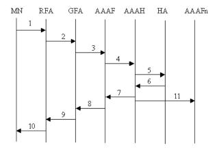
Fig. 5. Mobile IP Registration with Quasi-Registration
