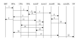
Fig. 6. Mobile IP Inter-handoff with Quasi-Registration
